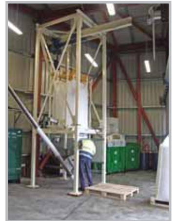
4. Bag loaded ready to discharge.
