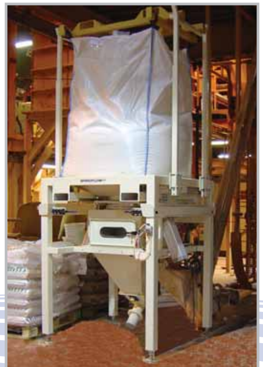
5. Bag loaded ready to discharge.
