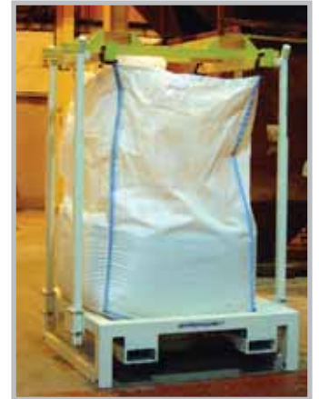
2. Loading bag into top frame.
