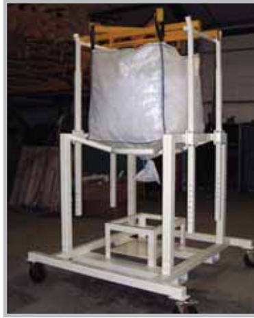
Customised Model T1 mounted on a wheeled frame that can also be moved by a forklift truck.
