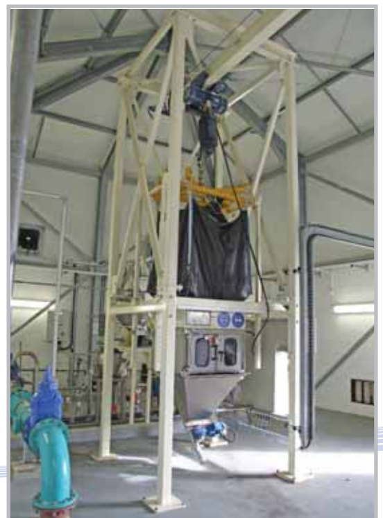
4. Bag loaded ready to discharge.
